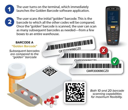
Each scan is compared to the same data content as the original "golden" barcode. If it matches, the display turns green with a positive match tone. If the scanned code does not match the "golden" barcode, the display will turn red with a negative beep sound.
